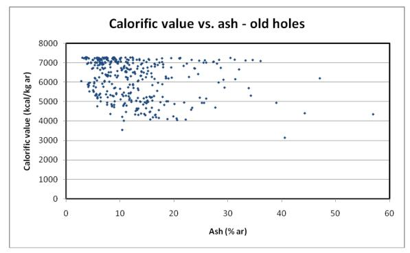
Figure 19.1 - Comparison of Correlation between Ash and Calorific Value between "Old" and "New" Holes
