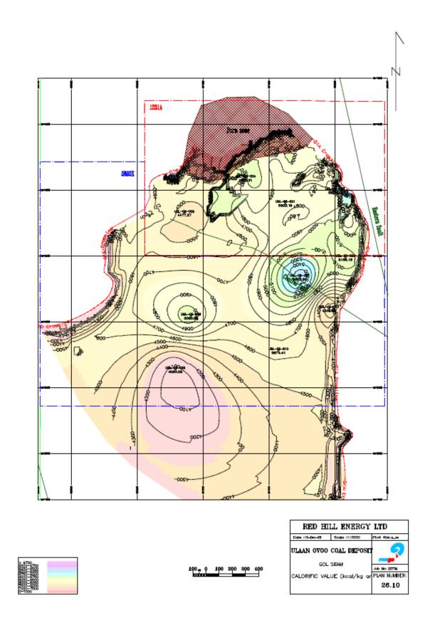
Figure 26.10 - Gol Seam Calorific Value (kcal ar) Isopachs
