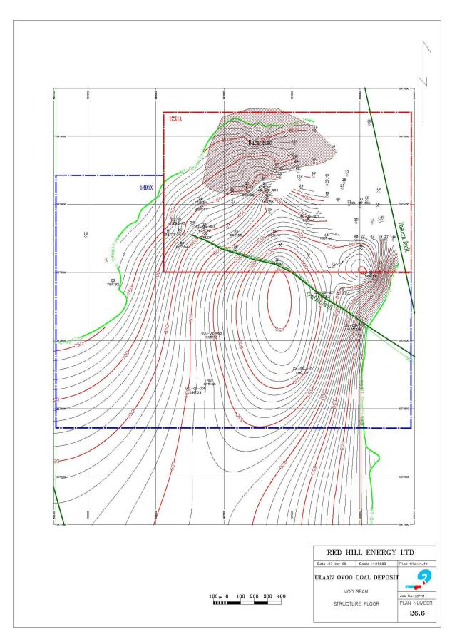
Figure 26.6 - Mod Seam Structure Floor
